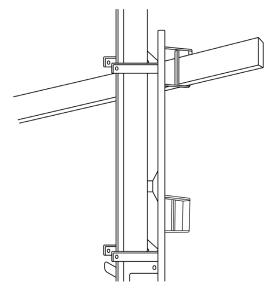
Once one side of the WorkSafe Aluminum Guardrail (#470645-E) is through, slide the WorkSafe Guardrail Carriage (#470625) onto the WorkSafe Aluminum Guardrail (#470645-E) with O-Ring facing down. Once the carriage is on the quardrail, slide the other end of the quardrail through the other top pump jack bracket rung.
