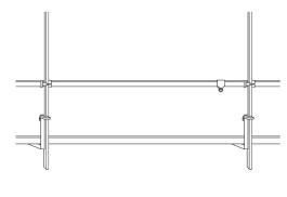
Once you have adjusted the pump jack system to working height, connect the WorkSafe Self Retracting Lifeline (SRL) (#470670) to the WorkSafe Guardrail Carriage (#470625) and your harness.
