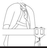
Install adjustable WorkSafe Telescoping End Stops (#4706300) to each end of the Guardrail. Adjust End Stops to length and depth of work surface. Locate and install end stop pins on Guardrail nearest to each outer pole rail.
